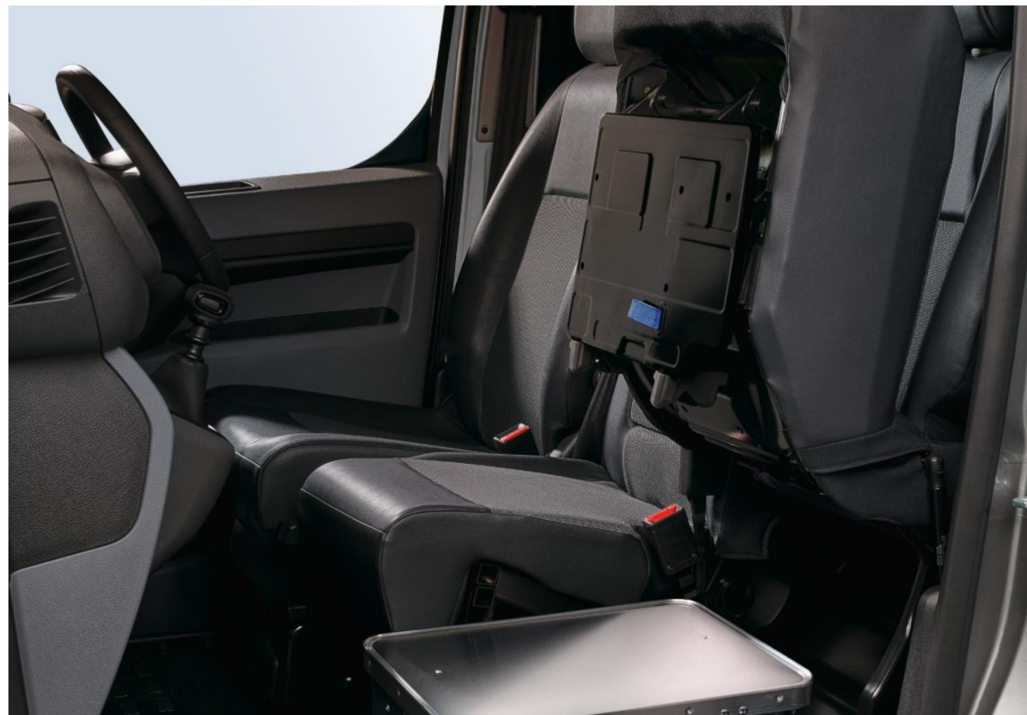
Load-through hatch within bulkhead.
